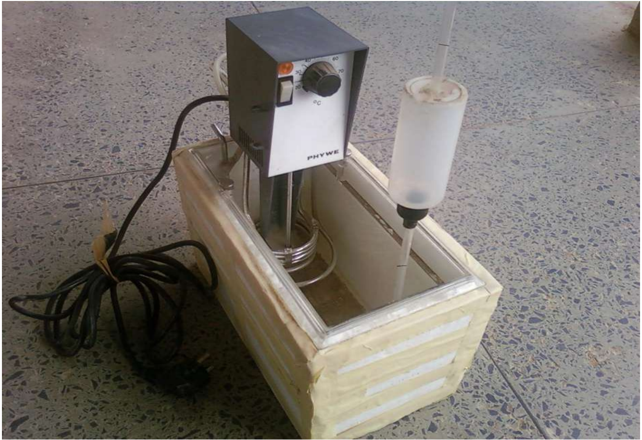
Picture 2: Plate I Photograph of the Constructed Temperature Control Viscometer
