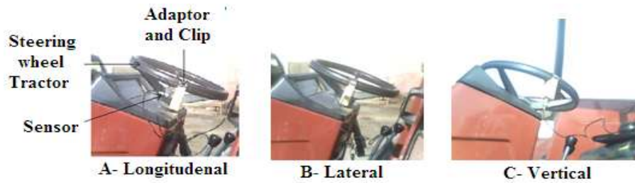
Figure 6 Accelerometer (Sensor) Locations on Steering Wheel During Measurement
